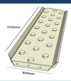
Floating Wetland unit shown with standard dimensions and modular planting cell layout.
